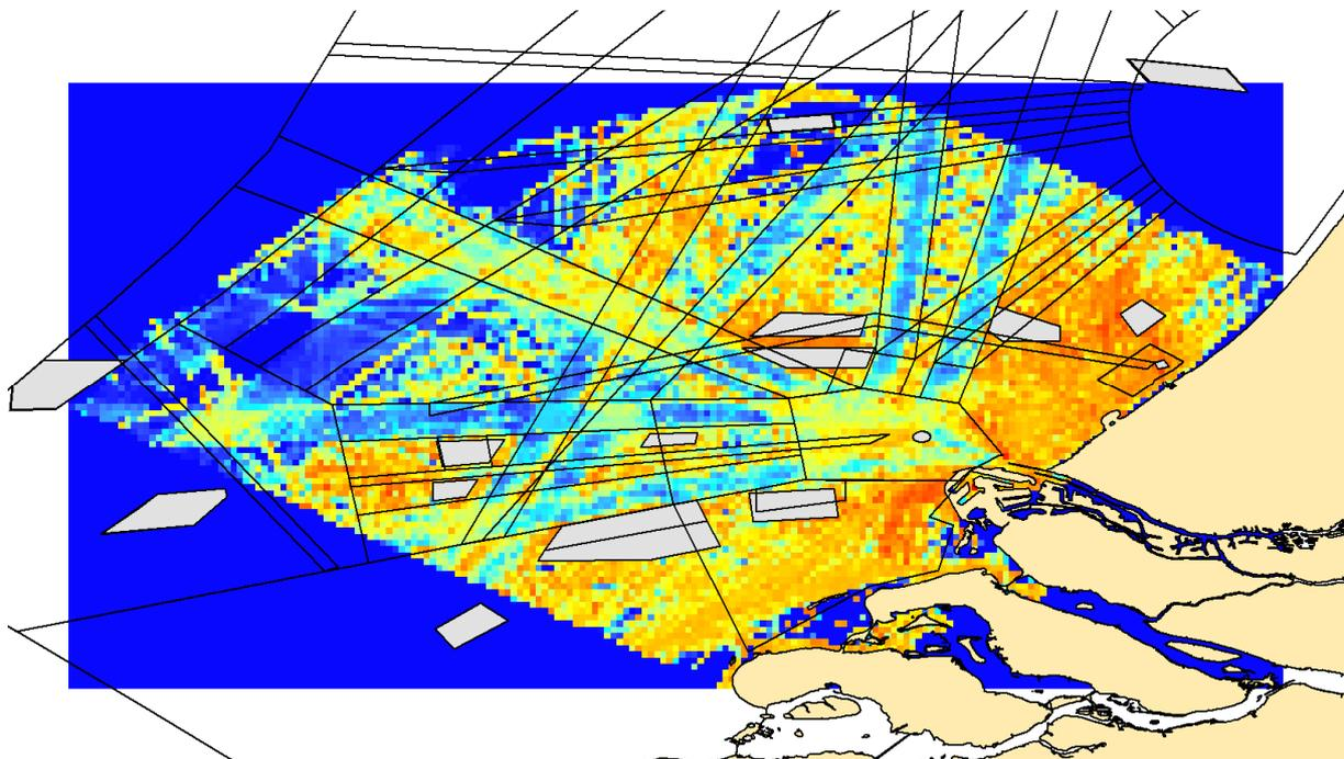
Figure 5. Example of statistical information (standard deviation of course over ground, based on coastal radar and AIS) near VTS Rotterdam, The Netherlands. Here we see that the course over ground in the shipping lanes is much more homogeneous than for instance in areas directly off the coast. Geographical information: Rijkswaterstaat Noordzee.
