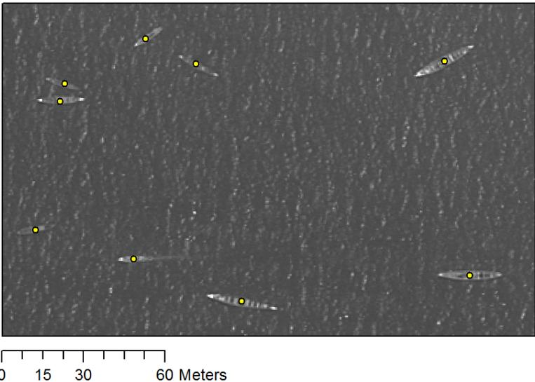
Figure 2. Example of small vessel detection off the coast of Mbour, Senegal. The yellow dots represent the detected vessel centres-of-gravity. Satellite image: © GeoEye, Inc. (2012), provided by e-GEOS S.p.A. under GSC-DA.
