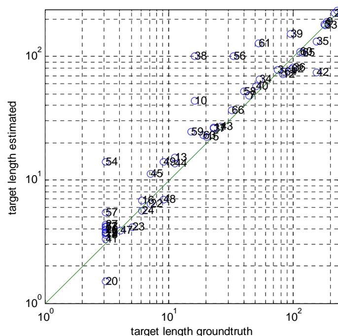
Figure 3. Estimated target vessel length against true target vessel length, based on robust segmentation, ship-wake separation, and length estimation; applied to optical images of the North Sea off the coast of Rotterdam, The Netherlands. Produced using products © GeoEye, Inc. (2011), provided by e-GEOS S.p.A. under GSC-DA.
