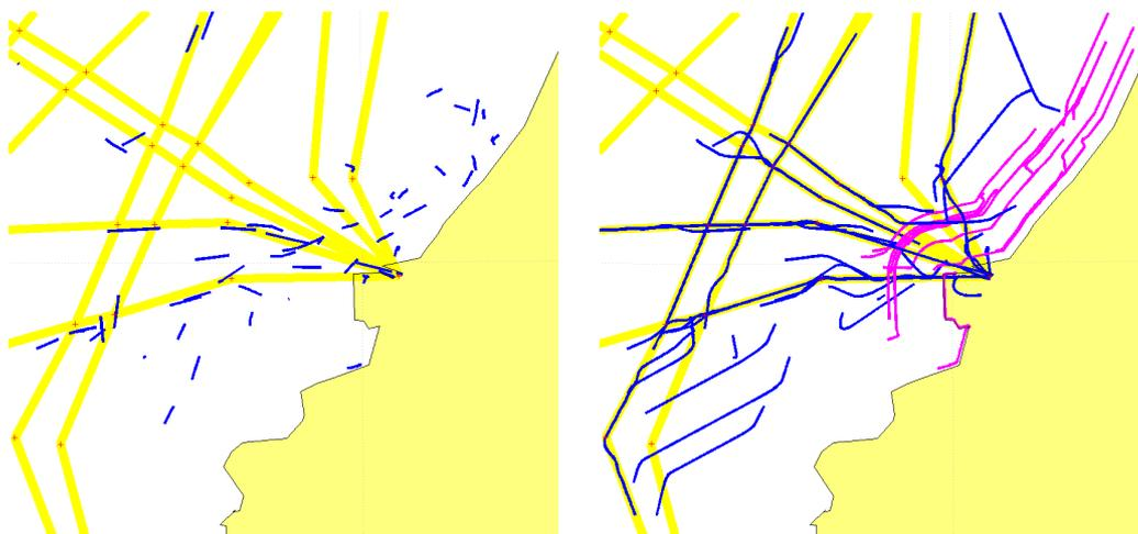
Figure 4. Prediction of vessel tracks over 2 hours (right) based on 10 minutes of data (left) of VTS Rotterdam, The Netherlands. The smaller vessels (magenta tracks) follow the coastline, whereas the larger vessels (blue tracks) follow the shipping lanes.
