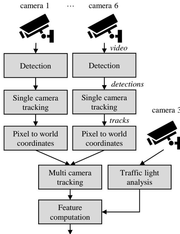
Figure 1. System architecture of the measurement method for objective cyclist behavior parameters
