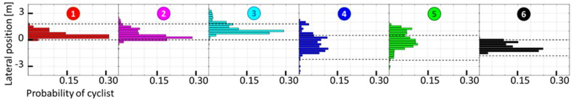
Figure 6. Lateral position of the cyclists on the cyclist path for the 6 camera's. The dotted lines show the borders of the cycle path.
